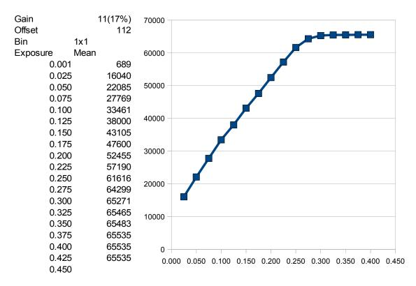
• We can see the roll into saturation occurs very nice and is not prolonged over an extended range because of the 5% gain increase. Also the drop in gain still leaves the minimum exposure of 0.001 second well above 0 ADU.
